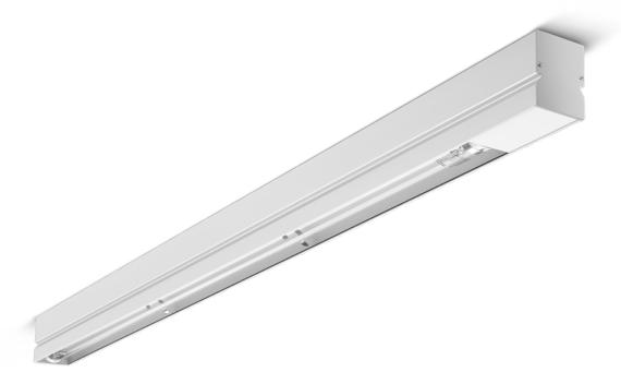
Antilia A-69-UV-Care is a professional ceiling and wall mounted luminaire for disinfection of the air and surfaces with ultraviolet radiation, for easy installation at the ceiling or a wall, with an adjustable light angle due to knobs on the sides of the enclosure. Available in two lengths (75cm and 135cm) and three power options (18W, 40W and 80W).
